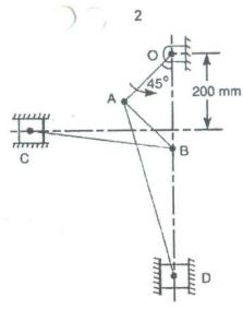
2. In the mechanism shown in figure, the slider C is moving to the right with a velocity of 1 m/s and an acceleration of 2.5 m/s². The dimensions of various links are AB = 3 m inclined at 45° with the vertical and BC = 1.5 m inclined at 45° with the horizontal. Determine (a) the magnitude of vertical and horizontal component of the acceleration of the point B and (b) the angular acceleration of the links AB and BC. (20)
